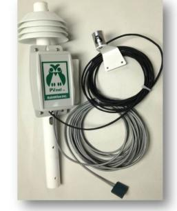
The new RainWise designed Amplified Silicon Pyranometer matches or exceeds the performance of the leading vendors of similar technology. The pyranometer's output amplification (0-2.5Volt) makes it's values easier to integrate. (*Note: Amplified Pyranomters are generally 25% more expensive than the standard non-amplified models, increasing the value of this station dramatically.*)
